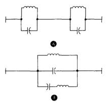
As previously described, one series-tuned circuit can again be replaced by a dipole to obtain a triband element. In **A** above, you then have two differently tuned, parallel-tuned circuits in series; in **B**, a series and a differently tuned parallel-circuit in parallel in the middle of the element. This "triband element" may be any Yagi-type radiator, director, or reflector, the groundplane radiator, or a cubical quad element.
